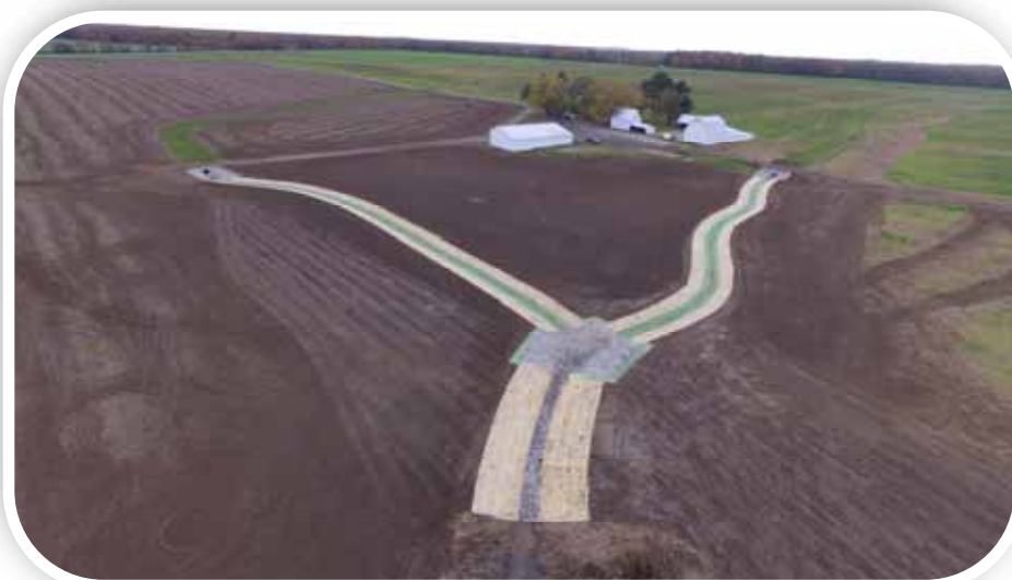
A birds-eye view of a large "Y" shaped grassed waterway with rock inlets and outlets cost-shared through the Maryland Agricultural Cost-Share Program (MACS).
