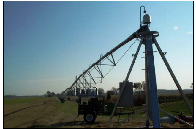
This is a center pivot irrigation system that was upgraded from hard hose through the EQIP program.
